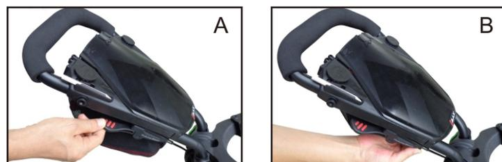
To engage the parking brake, rotate the hand brake lever mounted under the handle (A) towards the ground. The brake pin will extend into the wheel, locking the wheel in place. Rotate the brake handle upwards to unlock the brake. You can adjust the tension of the brake by turning the level barrel adjuster (B) counter clockwise to tighten, clockwise to loosen.
