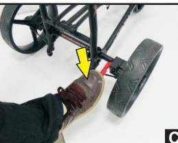
**4** Press the brake pedal to engage the brake.(A)
